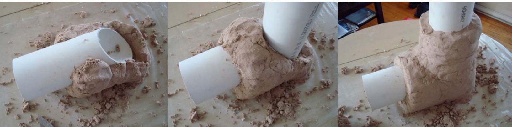
Figure 8: process of making the Holey Rokat using plastic pipes to make briquettes
