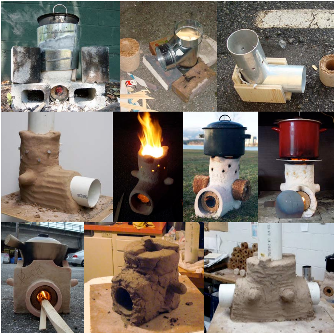
Figure 9: overview on the prototyping process of the Holey Rocket type. Following from top left: 1. A functional improvisation model at Aprovecho Stoves Camp, 2008. 2. A ready-made combustion chamber from a ventilation pipe. 3. An aluminium mock-up of the 'elbow' design. 4. A clay/sawdust model with plastic pipes; 5. The same model in action. 6. Briquette holders provide dry and warm briquettes before burn; 7. The front door provide a simple but efficient fire-volume manipulation. 8. Introduction of the rocket principle to WWF's Mdula stove. 9. A thicker-wall version of the stove for slow-burn performance and improve heat transfer to the pot with a wider top rim. 10. An attempt to test double feed with inserting two briquettes from opposite sides to improve the heat output
