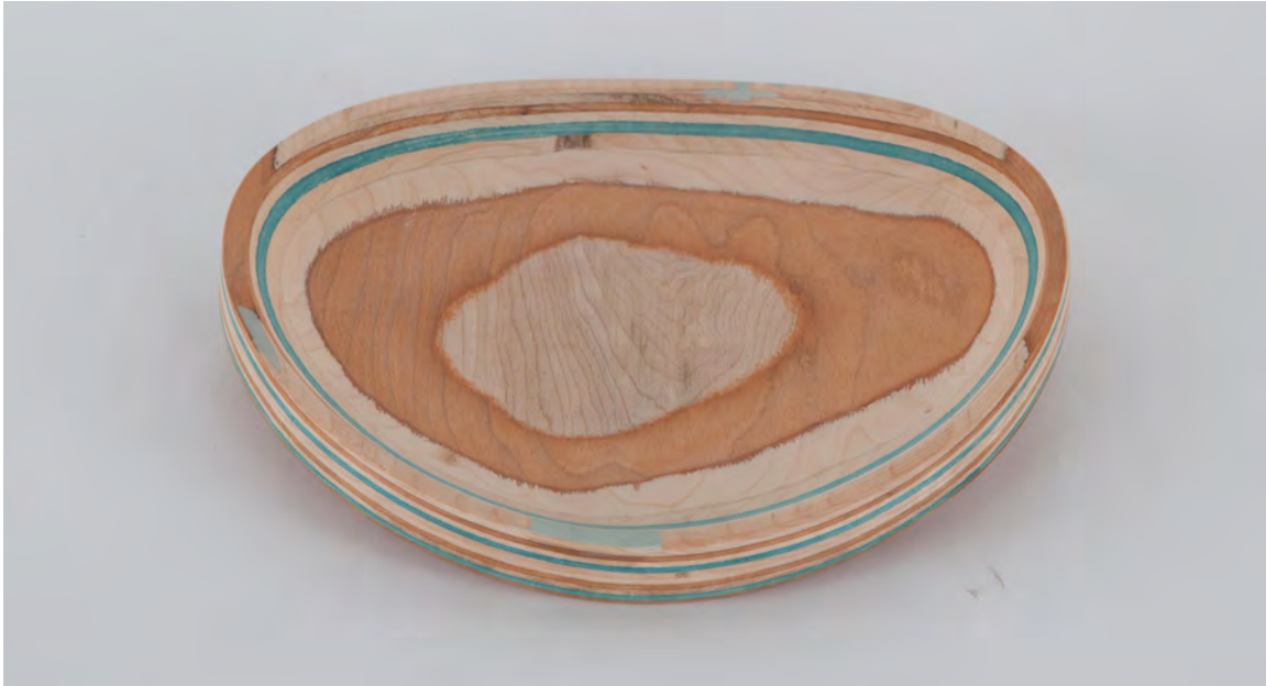
Figure 3. Bent lamination plate, wood veneer with Bondo repair
