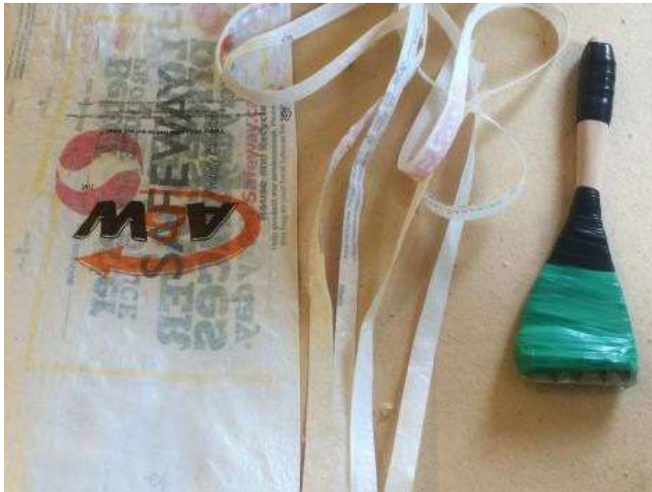
FIGURE 4: Jay Havens. The Bear Claw with Rollback Rawhide made into ribbons . 2016. Wooden spatula, razor blades, electrical tape, hot glue. Splint making tool. Kariton Studio, Abbotsford BC. Photo by Jay Havens. Used with permission.
