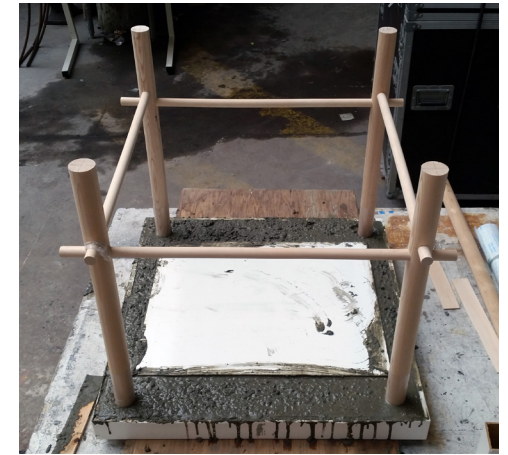
Fig. 47. STÖN Process 14. In an effort to make the concrete component of the STÖN lighter, a 20mm Melamine panel was used to create a void in the underside of the table's surface. (Photograph by M. Harkness, 2017)
