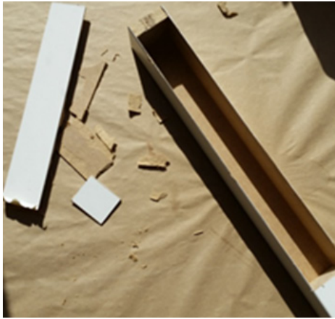
Fig. 4. IKEA LACK Dissection (Photograph by M. Harkness, 2016)
