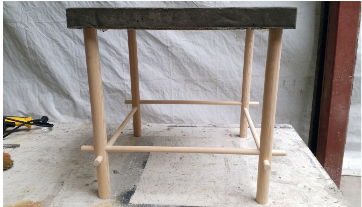
Fig. 49. STÖN Process 16. The thin, particle board edges of the LACK mold are easily peeled away from the concrete top of the STÖN table. (Photograph by M. Harkness, 2017)
