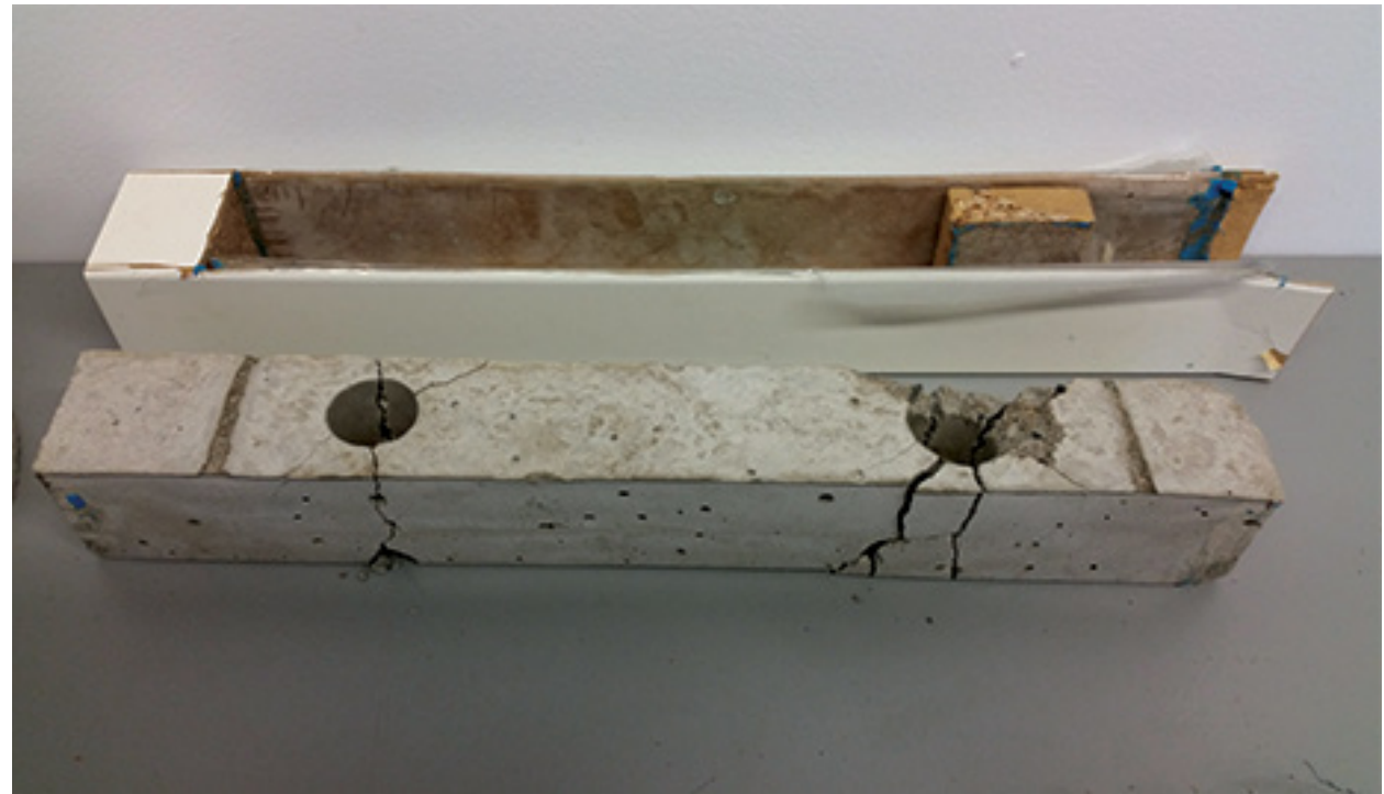
Fig. 56. Wall Hanger Process 6. The distance from the wooden coat peg to the edge of the LACK mold was too small. Presumably, this made the Wall Hanger fail as it was removed from the mold. (Photograph by M. Harkness, 2016)
