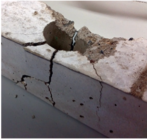
Fig. 55. Wall Hanger Process 5. Detail of the failed Wall Hanger. (Photograph by M. Harkness, 2016)
