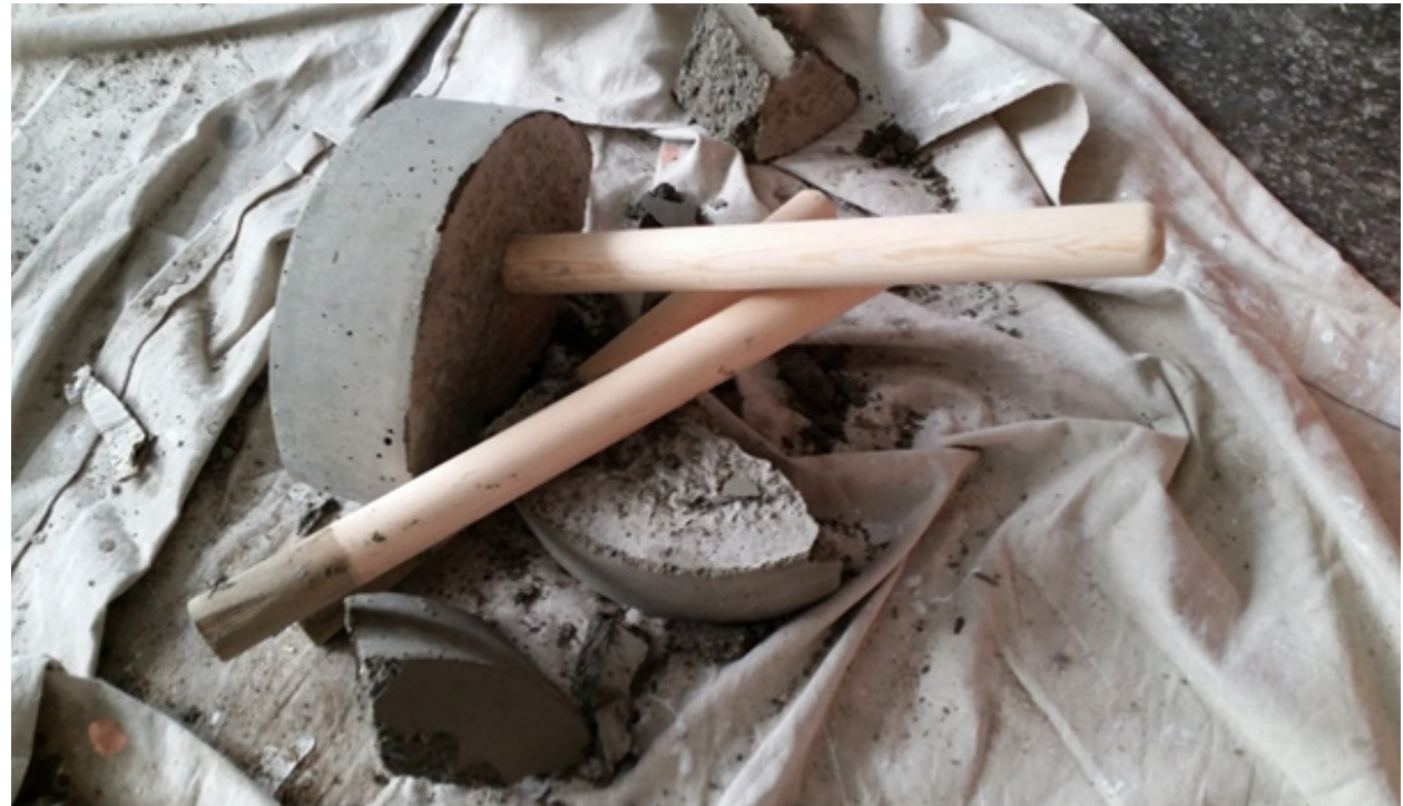
Fig. 33. One of Many Failed KRÄFTIG Stools. This image shows a KRÄFTIG that broke as it released from the mold. If the KRÄFTIG's legs are positioned too close together when stuck into the concrete, the stool can become weakened. (Photograph by M. Harkness, 2016)
