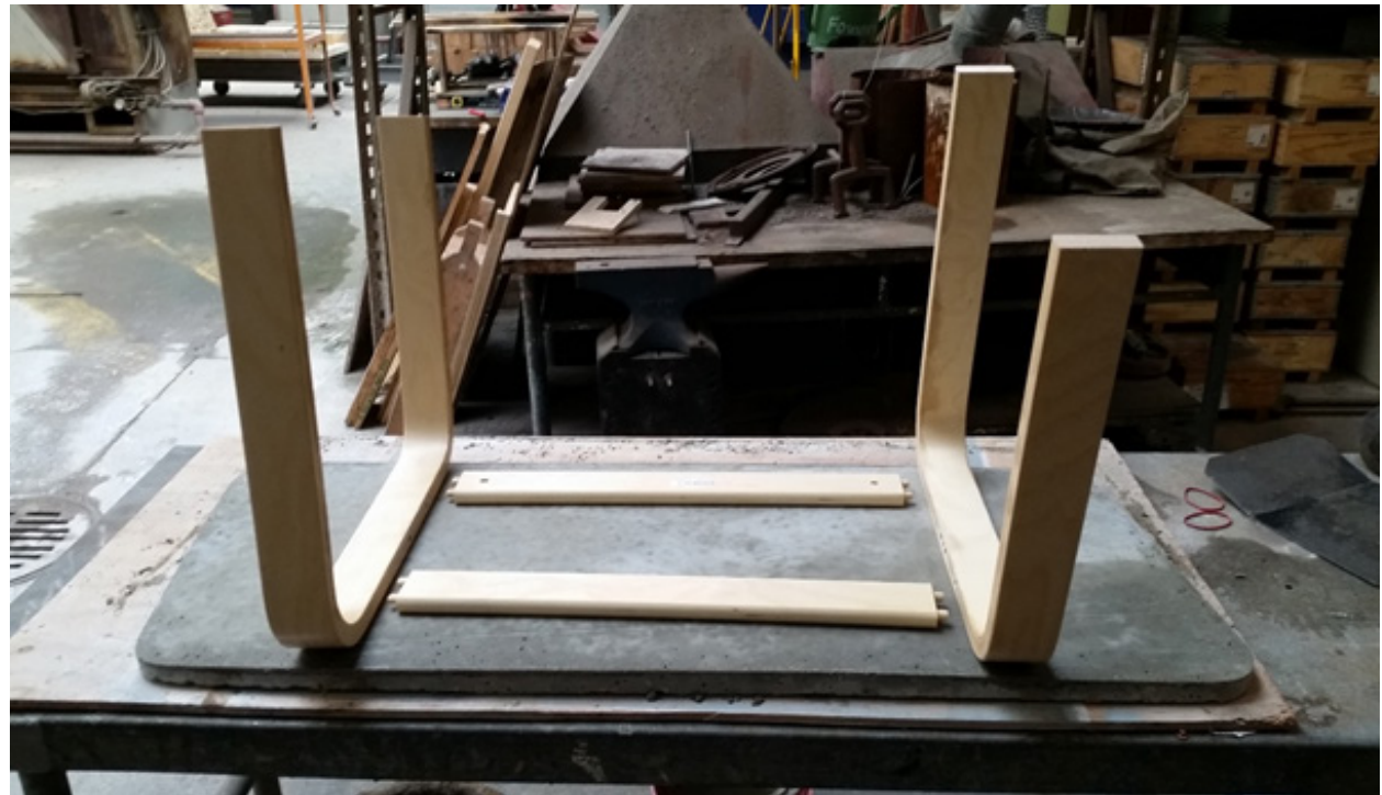
Fig. 72. Coffee Table Process 8. The wooden base of the table is then created using the PELLO Armchair's pre-drilled holes and fastener's. All that is left to do is to trim the two long sides of the legs using a hand saw. (Photograph by M. Harkness 2016)
