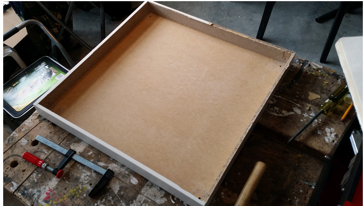
Fig. 41. STÖN Process 8. The completely hollowed out LACK table top can now be used as a mold. (Photograph by M. Harkness, 2017)
