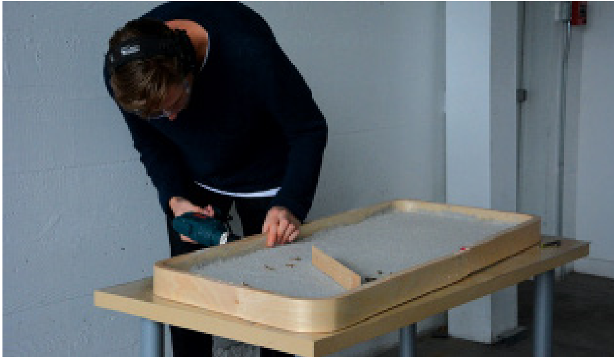
Fig. 69. Coffee Table Process 5. Disassembling the mold after the concrete has dried. (Photograph by M. Harkness, 2016)
