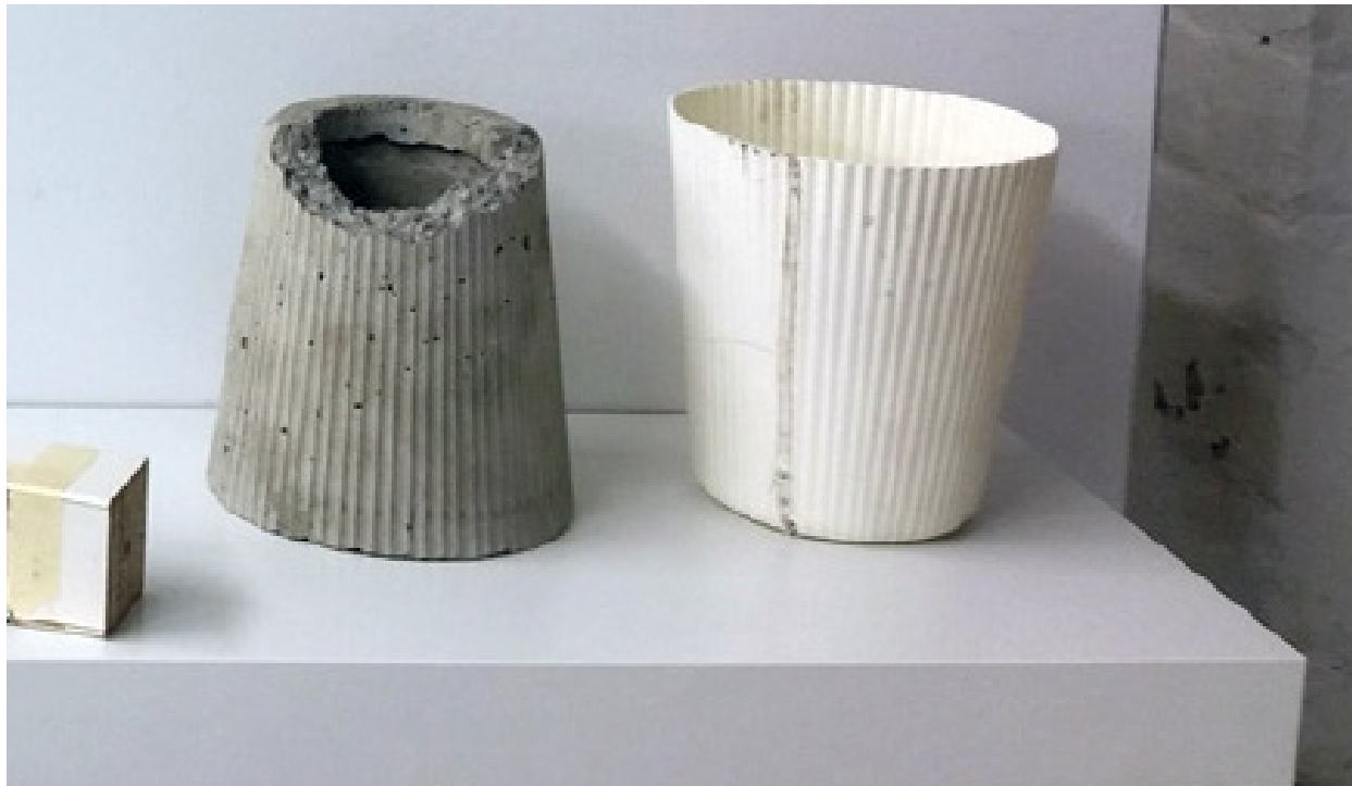
Fig. 50. Lamp Process 1. A failed lampshade beside its NEJKON plant pot mold. (Photograph by M. Harkness, 2016)
