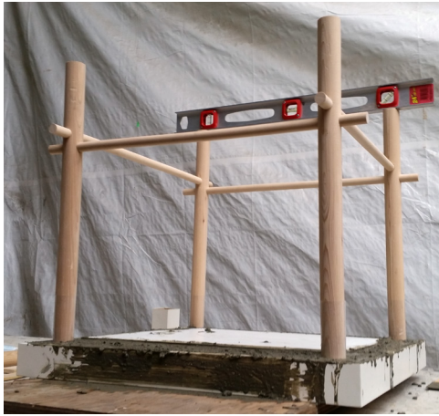
Fig. 48. STÖN Process 15. Once the STÖN's frame is stuck into the wet concrete a spirit level ensures the furniture object will be level once the concrete has dried. (Photograph by M. Harkness, 2017)
