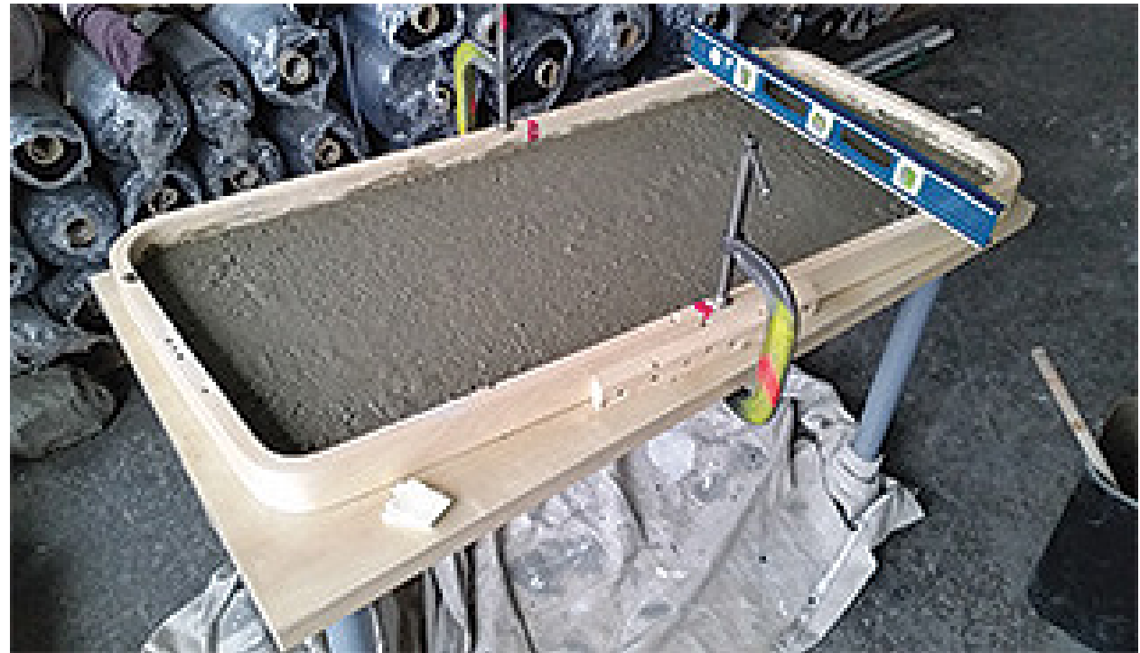
Fig. 68. Coffee Table Process 4. With the PELLO frame clamped down to the work surface, the concrete is poured. (Photograph by M. Harkness, 2016)
