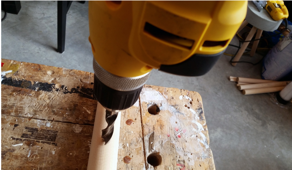
Fig. 42. STÖN Process 9. Drilling through the dowel to create the STÖN frame. (Photograph by M. Harkness, 2017)
