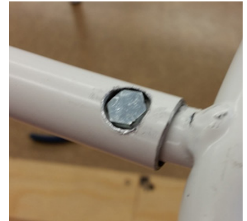
Fig. 62. Chair-Table Process 6. The ADDE Chair frame is then put back together using the existing IKEA fasteners, and rubber clips hold the concrete top in place. (Photograph by M. Harkness, 2016)
