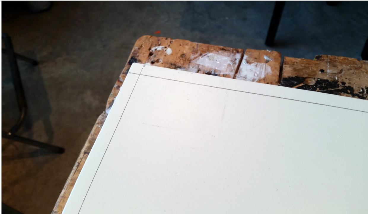
Fig. 34. STÖN Process 1. Measuring out 9mm from each edge of the LACK table top. (Photograph by M. Harkness, 2017)
