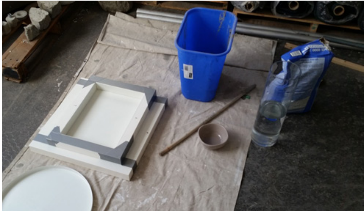
Fig. 8. Preparing to Mix the Concrete. Concrete mixing tools: A level work surface, a bag of concrete mix, a bucket to mix the concrete and water in, a few liters of water and a sturdy mixing stick. (Photograph by M. Harkness, 2016)
