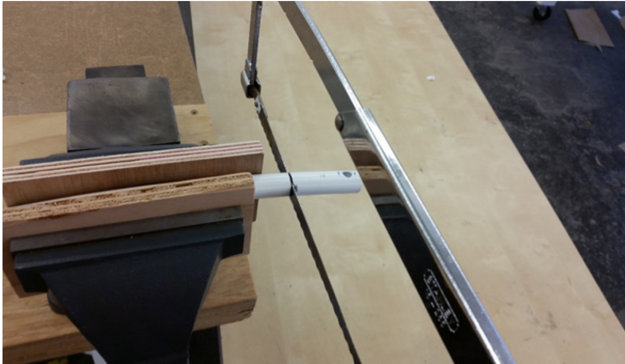
Fig. 61. Chair-Table Process 5. Using a hacksaw, the ADDE Chair Rails can be cut shorter to fit the newly formed concrete top. (Photograph by M. Harkness, 2016)
