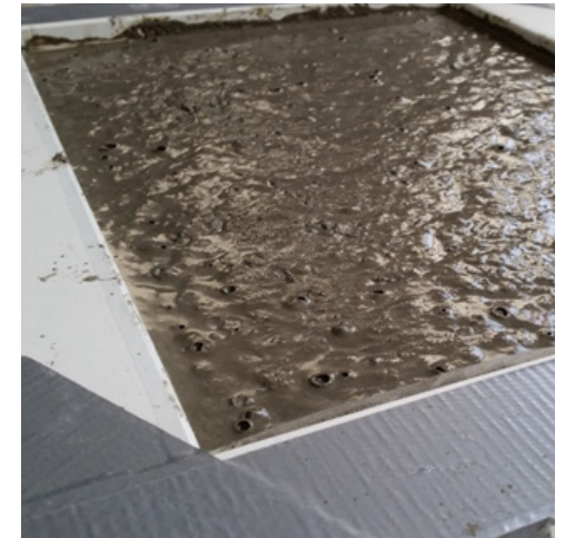
Fig. 9. Freshly Mixed and Poured Concrete. Once thoroughly mixed and poured into the mold, the concrete can be aerated by repeatedly tapping the edge of the mold with mixing stick to release any trapped air bubbles. (Photograph by M. Harkness, 2016)
