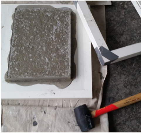
Fig. 10. Concrete Component Released from the Mold. Although not required, a rubber mallet helps release the concrete from the mold. Any concrete that seeped out from the bottom edge of the mold is fragile and is easily cleaned off. (Photograph by M. Harkness, 2016)
