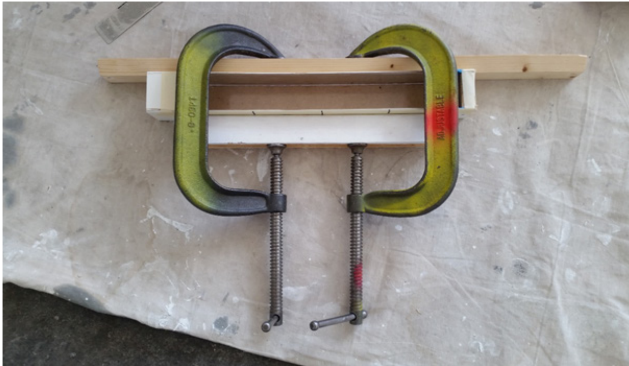
Fig. 53. Wall Hanger Process 3. The LACK's thin MDF walls are reinforced using G-Clamps and wood cauls. This clamp pressure prevents the wet and heavy concrete from bowing out the sides of the mold. (Photograph by M. Harkness, 2016)
