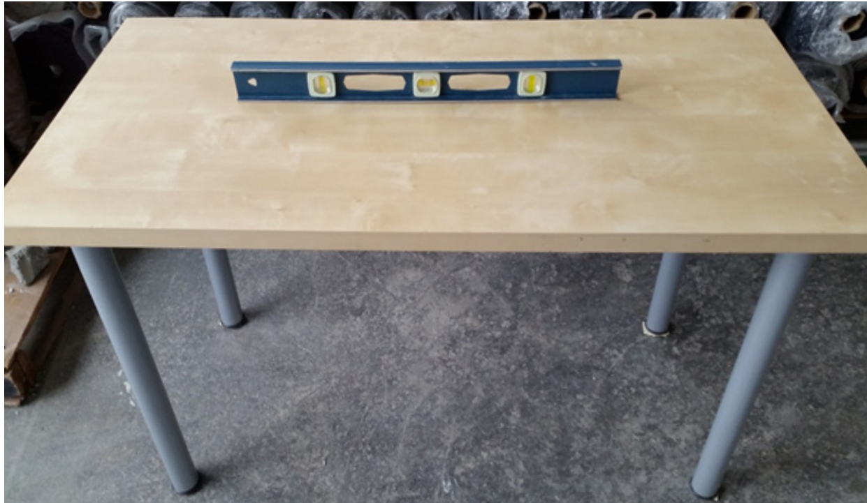
Fig. 65. Coffee Table Process 1. Choosing a smooth, level and, plastic-coated concrete pouring surface will significantly affect the finished table's top surface. (Photograph by M. Harkness, 2016)
