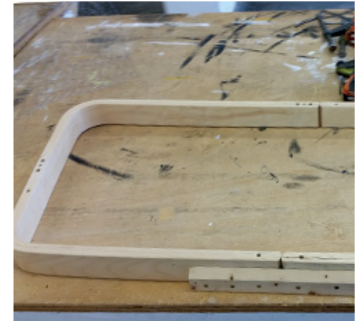
Fig. 66. Coffee Table Process 2. The curved legs of a PELLO armchair create the mold for the table. A piece of scrap wood can be nailed or screwed into the PELLO frame to connect each leg-end and complete the mold. (Photograph by M. Harkness, 2016)
