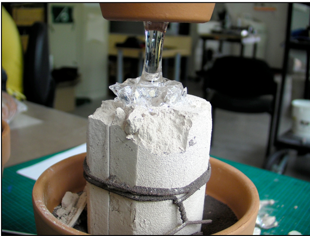
Figure 15: Glass casting setup, post-firing
