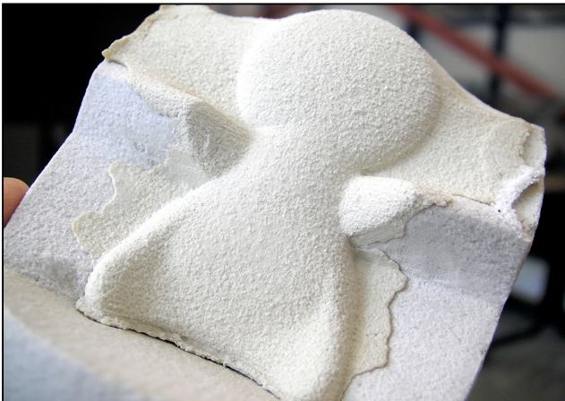
Figure 11: Printed mould and slip cast ceramic
