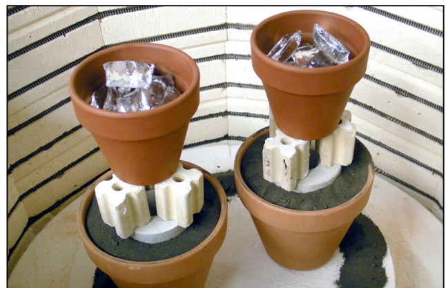
Figure 13: Glass casting setup, pre-firing
