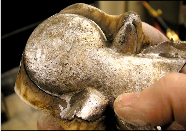
Figure 10: Printed mould and cast aluminum
