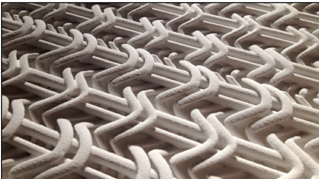
Figure 7: Unfired 3DP glass, open woven form
