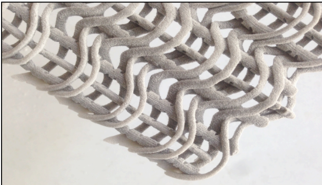
Figure 8: 3DP fired glass, open woven form
