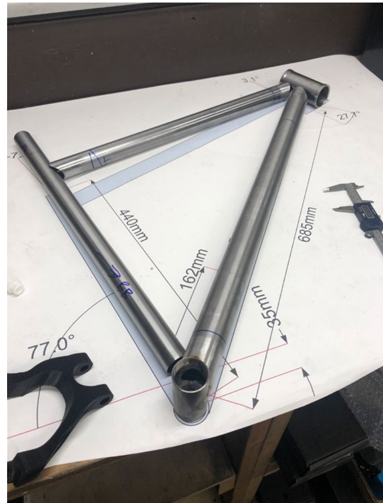
Fig. 45: Blueprints during the process of building the frame.
