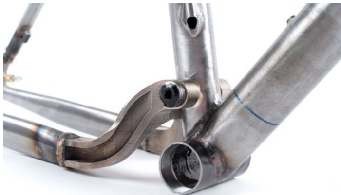
Fig. 50: Close shot of the pivot point and yoke of the frame.
