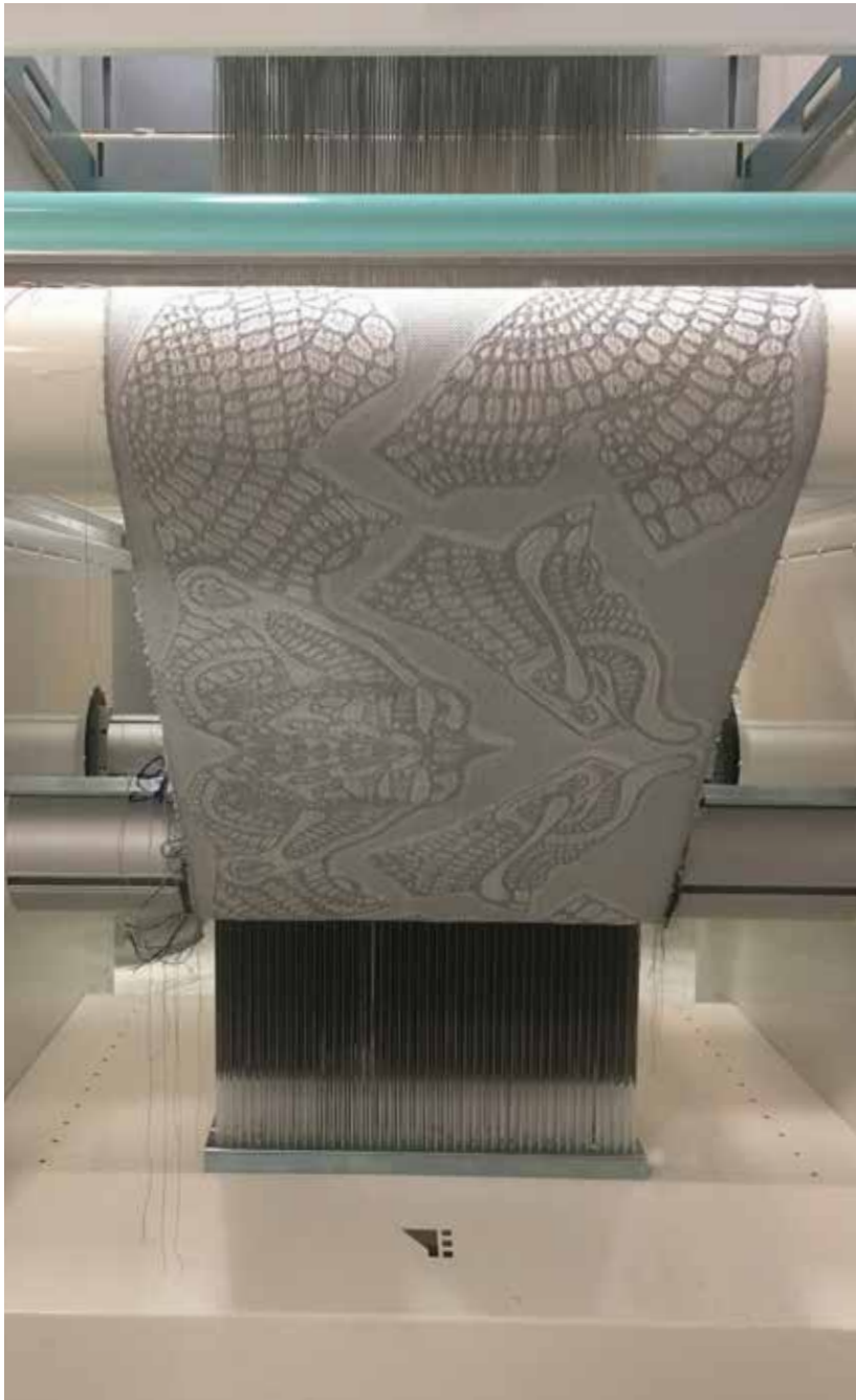
Image 69: Digital Jacquard Loom, Material Matters Research Center, 2019
