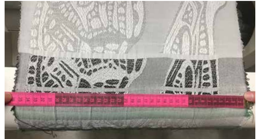
Image 59: Weave tests: Unbalanced, 2019
