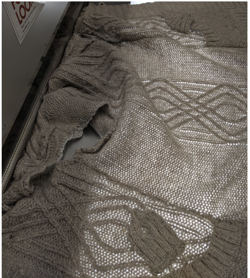
Fig. 35- First full sweater test in the felting machine. All toggles were removed and the sweater inserted as flatly as possible.
