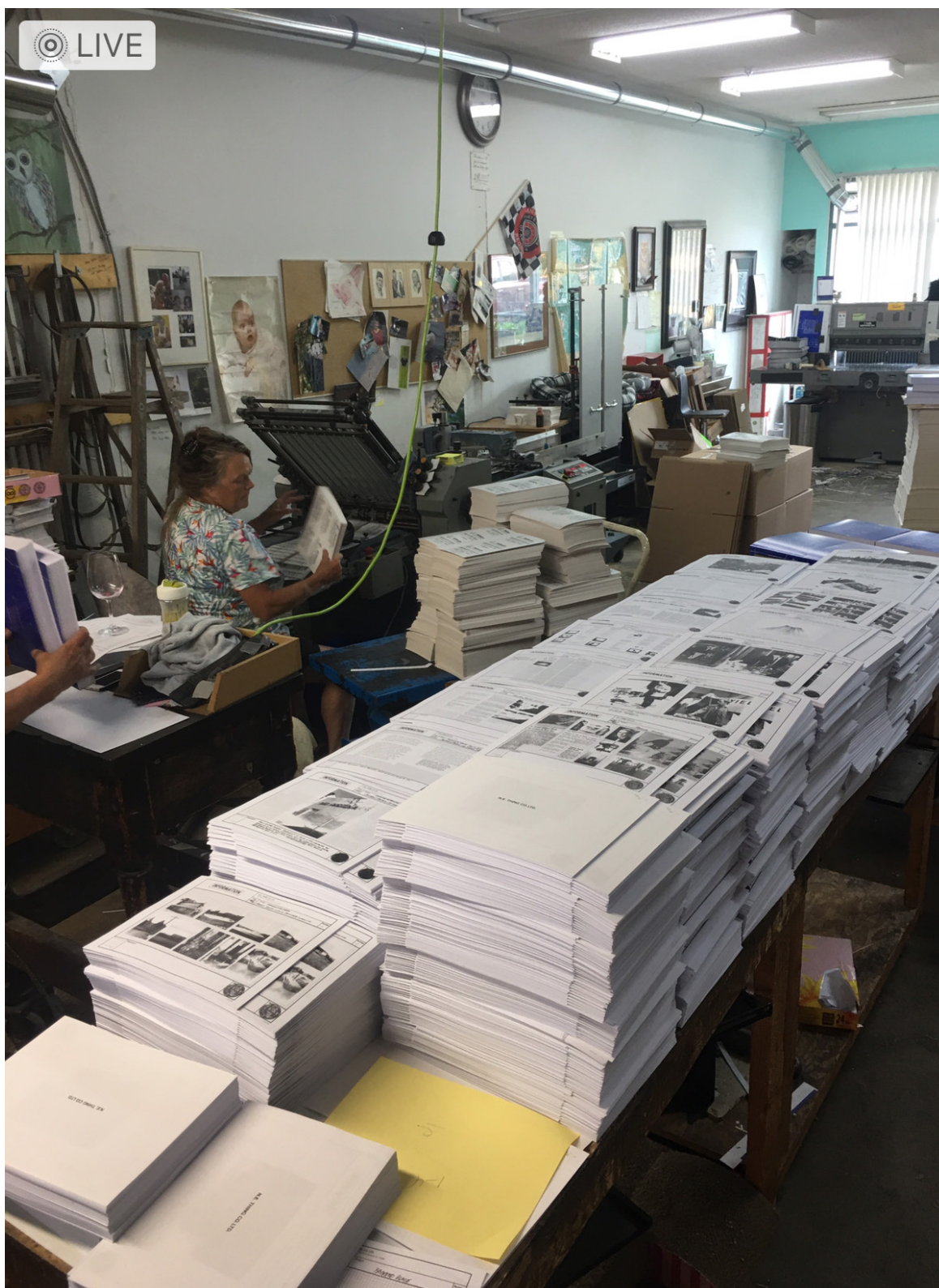
Figure 29. Roughly sixteen stacks of collated “sets.” Each set contains twenty-four consecutive pages, once “married,” (assembled) they will be put into an industrial perfect-binding (glue-binding) machine.
