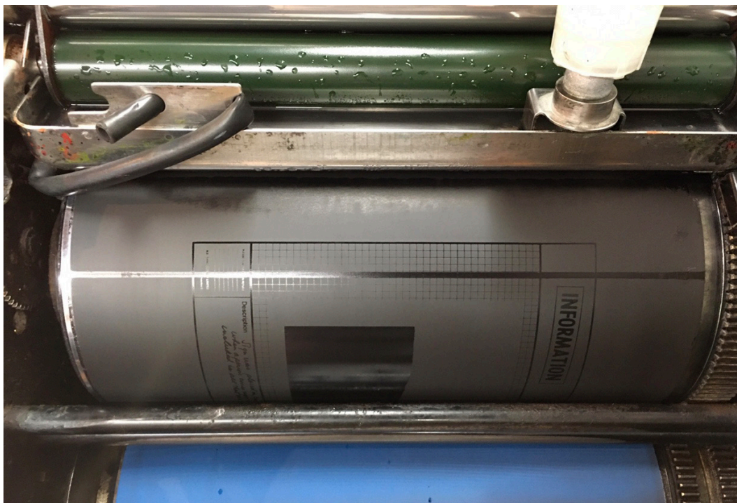
Figure 13. Roller-pressure check. The press rollers are inked up and “engaged” to the plate to determine if the lateral pressure is even. In this case, a successful test (note the even bead of ink across the printing plate).
