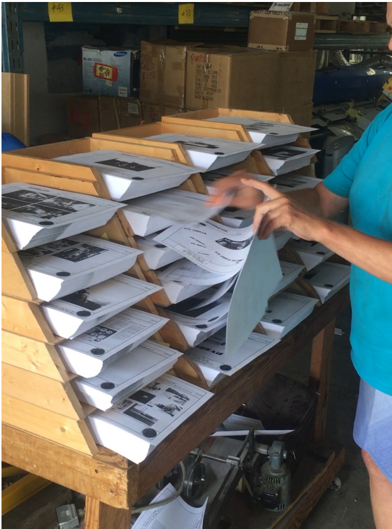
Figure 27. Video-still of a bindery expert collating twenty-four pages at a time by hand. This method required fifteen sets of full shelves of twenty-four pages x545 sheets to be paginated, nearly 200,000 lifts, aided only by a rubber finger slip. Hand-work of this nature is an efficient, yet difficult skill learned only with years of practice.
