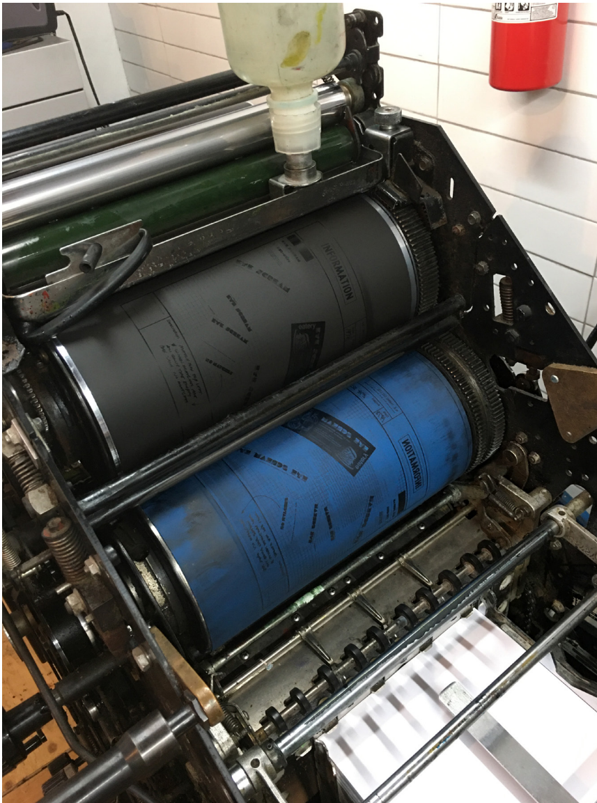
Figure 17. Pictured: water fountain, plate with inked positive image, blanket with negative image and paper feed mechanism. Image: Page from Companies Act documenting NETCO's restaurant, EYESCREAM.
