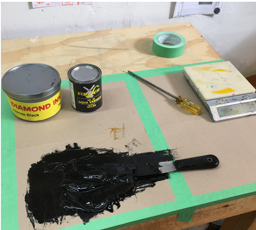
Figure 16. Ink, varnish and scale. The varnish has the consistency (and colour) of honey out of the fridge, requiring much effort to mix.
