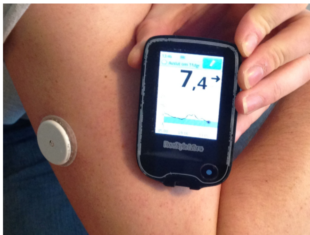
Figure 3: Continuous glucose monitor. 2016. Wikimedia commons, licensed under CC BY-SA 4.0
