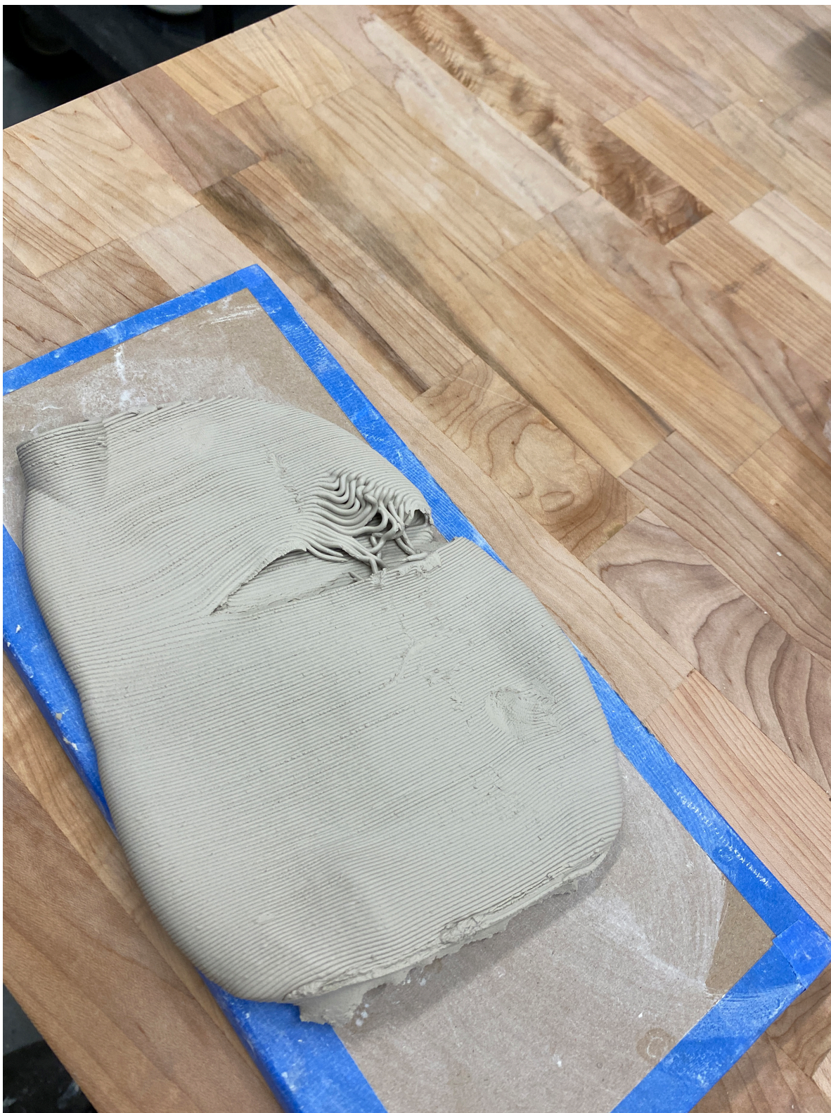
This happened a lot. Making a tall slender vessel was technically challenging. At this point I was learning how to balance the machines flow rate, print speed, nozzle size, and clay consistency. 2020. Avi Farber
