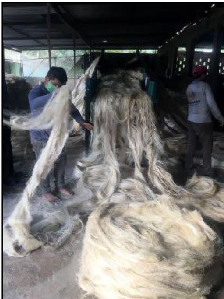
Fig. 8. Raw henequén being fed into cord/rope-making machines. 2021. Plantation Factory Cacalchén, Yucatán, Mexico. Photo: Andrea Hennig.
