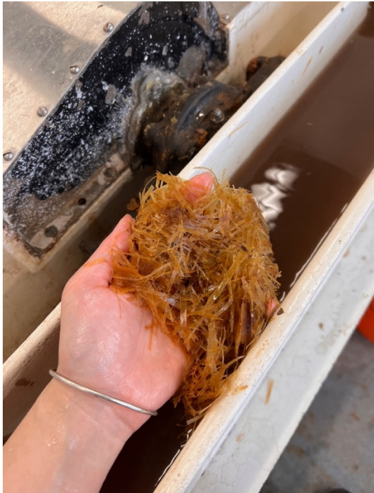
Fig. 14. After processing with the simmering in soda ash solution, the black cotton barks are then cut into small pieces and beaten in the paper Hollander beater for ninety minutes. The bark is not beaten into pulp form but remains in a rigid fibre structure. Photo courtesy of the artist.
