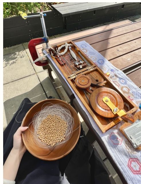
Fig. 22. The separated paper thread is spun onto a bobbin with a box charkha. Photo courtesy of the artist.
