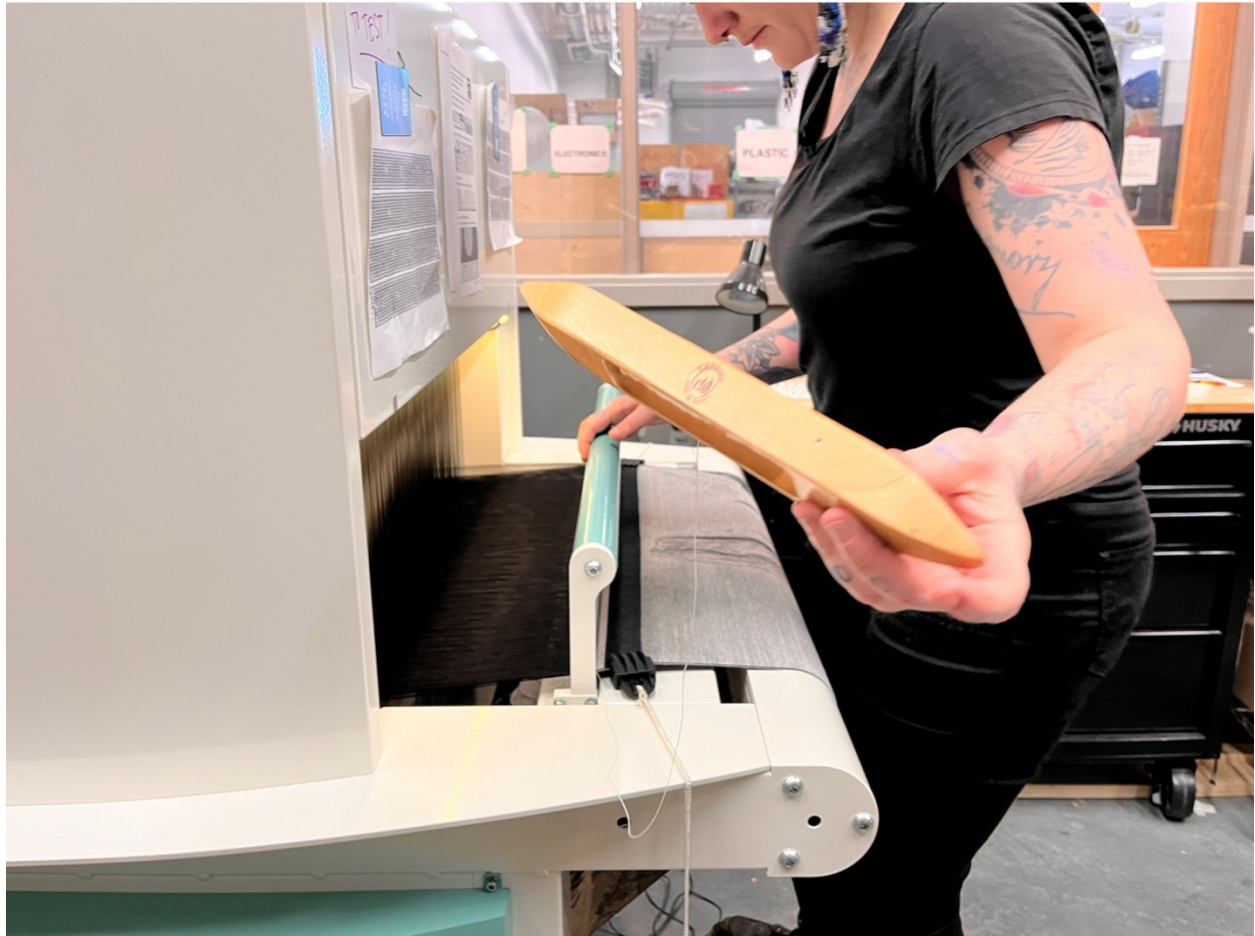
Figure 14: Weaving on TC2 Jacquard Loom. 2024.
